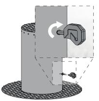
To unlock the electromechanical bollard, insert the key into the slot and turn in a clockwise direction.
